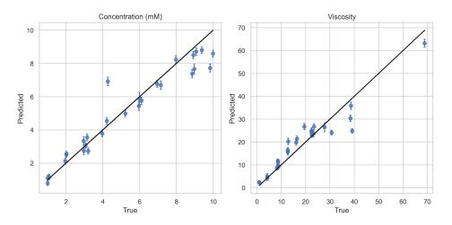
Figure 5: Prediction of the parameter of interest (concentration) and confounding variable (viscosity) with associated uncertainties. The error bars represent 99% uncertainty interval. The median prediction error of concentration is 0.33 mM. The solid black line in the plots indicates the true values.
