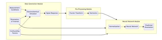
Figure 1: Detailed schematic of Phase 1 or pre-training phase - contains data generation module, physics-based processing module and a deep learning module.
